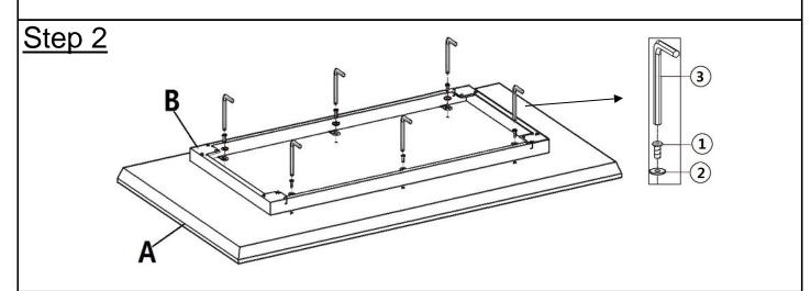
Carefully place the Table Top(A) facedown on a clean, non-marring surface. Attach the Metal Frame(B) to Table Top(A) using Bolts(①) and Washers(②) with Allen Key(③).
