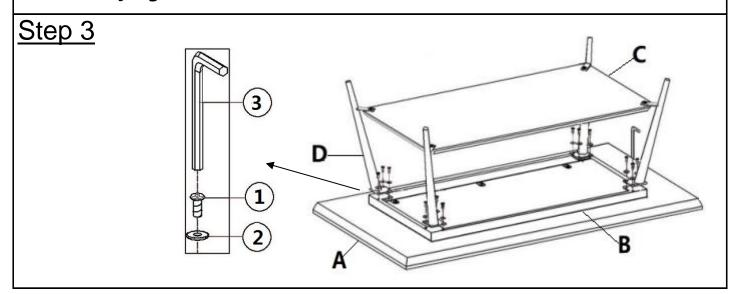
Attach the assembled Middle Board(C) and Legs(D) to Metal Frame(B) using Bolts(1) and Washers(2) with Allen Key(3).
