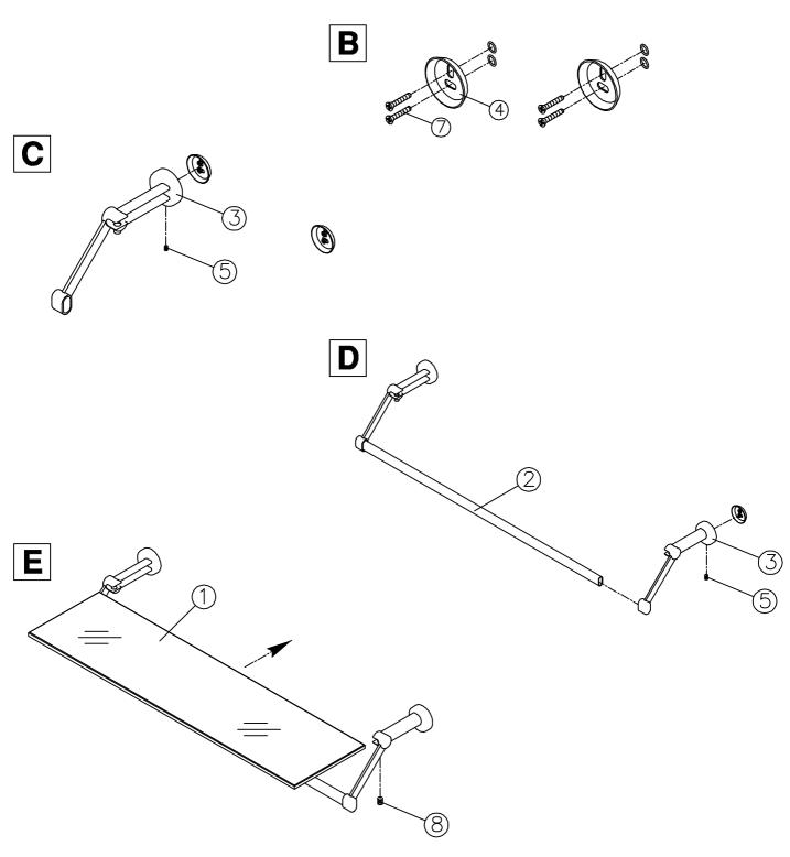
Please note: Part #8 (screw) should be loosened from part #3 (hinges) first before placing the glass shelf on hinges. After glass is settled, part #8 screws may now be tightened.
