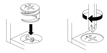
Turn cam lock clockwise to tighten.
