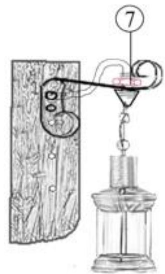
3 Wire the wires through the board to complete the assembly
