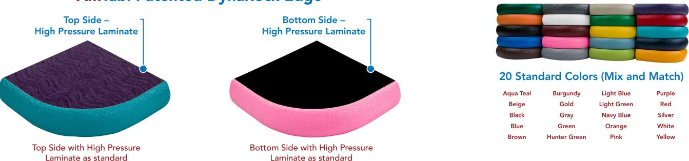
All cores shall be permanently bonded with a high pressure laminate top side and truly balanced with a high pressure laminate bottom side. Edges shall be sealed and protected with 100% solid polyurethane and permanently bonded to the table top. The truly balanced and hermetically sealed table tops are uniquely designed to prevent moisture from entering the core and promote anti-microbial sanitary surfaces after easy cleaning day in and day out.
