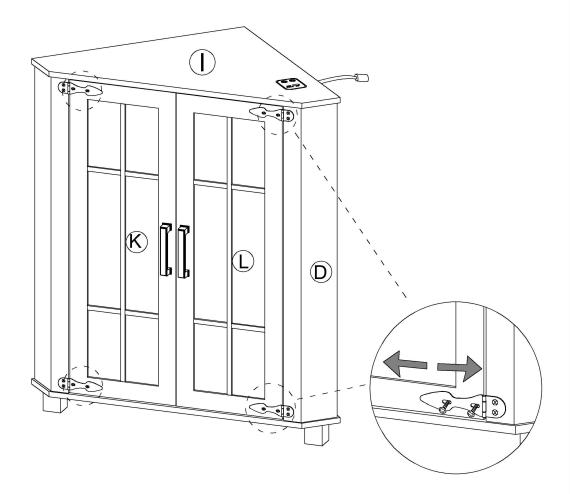
If there is a large gap after the installation of the door, please twist the screw of the door hinge back halfway and move the door left and right.
