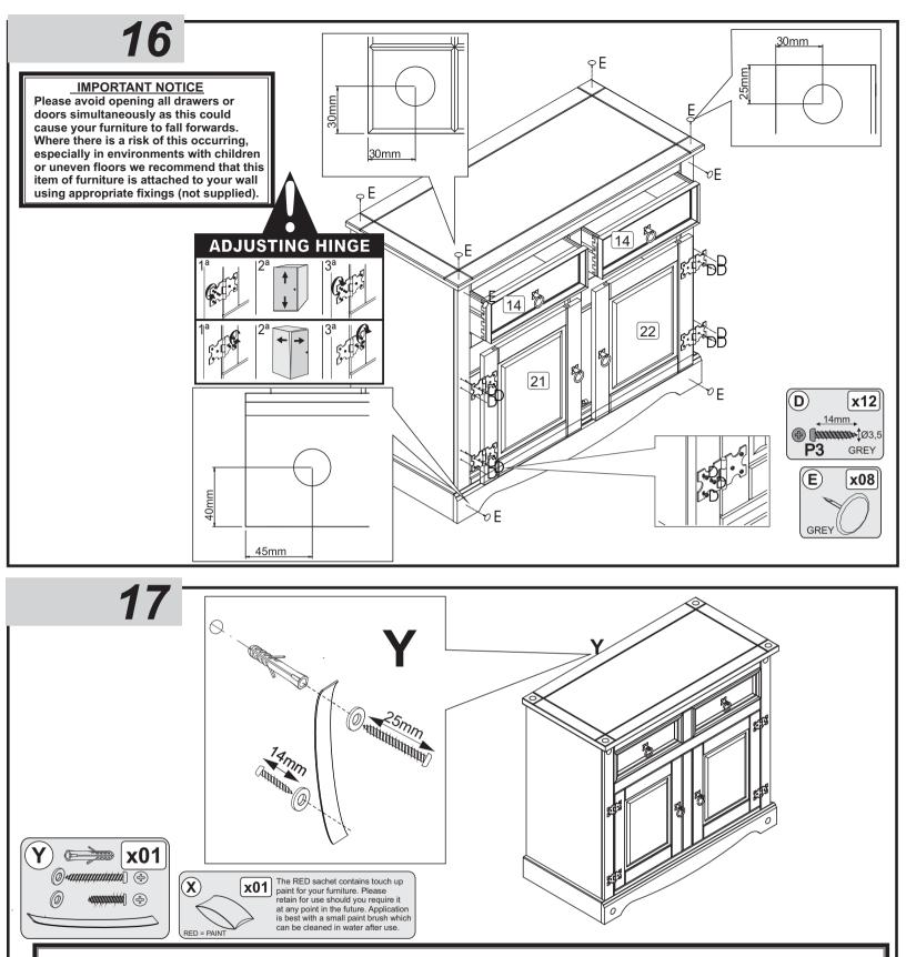
WARNING: CHECK FOR HIDDEN PIPES AND CABLES BEFORE DRILLING.
