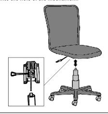
Before seating and using the chair for the first time, make sure that all screws are properly tightened.
