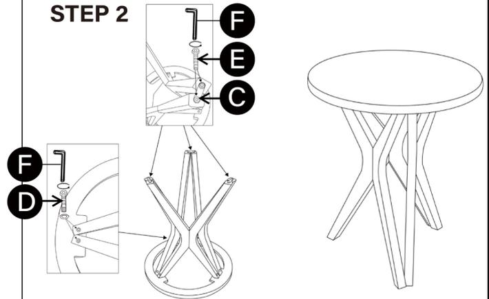
Use flat washer C and SHORTER screws E to attach the other end of the legs B together. Please make sure all bolts are fully tightened before using.
