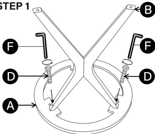
Attach legs B to table top A using LONGER screws D as shown above.
