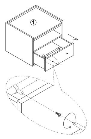
Un-screw the pre-installed handles inside the drawer.
