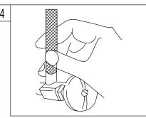
4. Turn on water supply valves and check for leaks, especially at hook-ups to supply lines.
