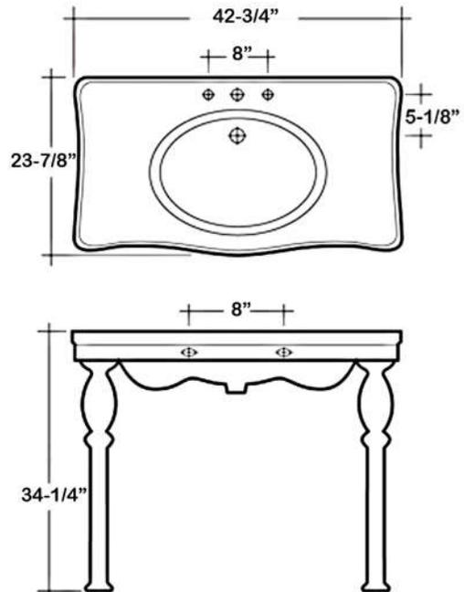
Dimensions of fixture are nominal and may vary within the range of tolerances established by ASME Standard A112.19.2.2013. Dimensions and specifications subject to change without notice.
