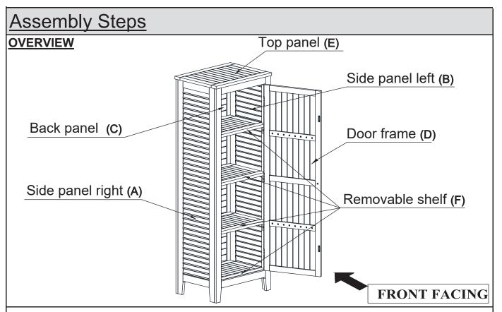
This Cabinet has multiple parts and may require up to 45 minutes to assemble. To give you an overview of the Cabinet parts, we've provided the above picture to put the various parts in perspective. Please read through the instructions below to familiarise yourself with the parts and steps before assembly.
