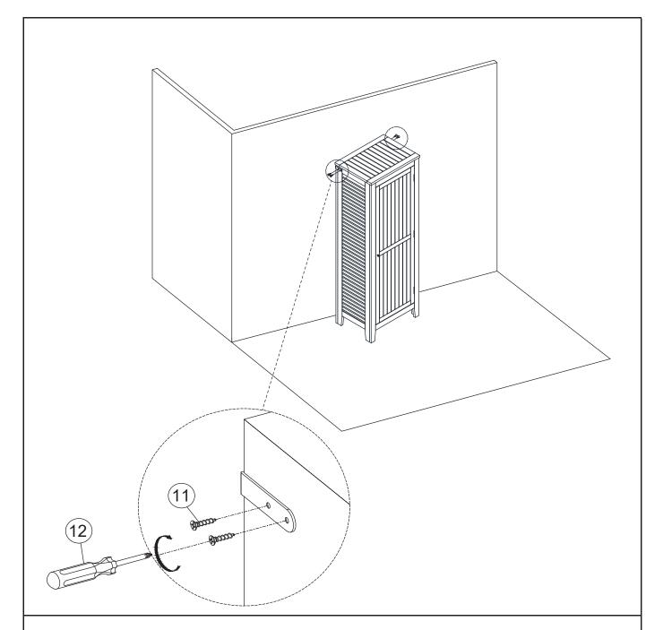
D: Move the Cabinet against the wall. Then connect the L-shaped Metal Bracket (7) to Cabinet position in the wall using the Self Tapping Screws (11) and Screwdriver (12)(not provided), as shown above. The Cabinet Restraint Device is now installed and is ready for use.
