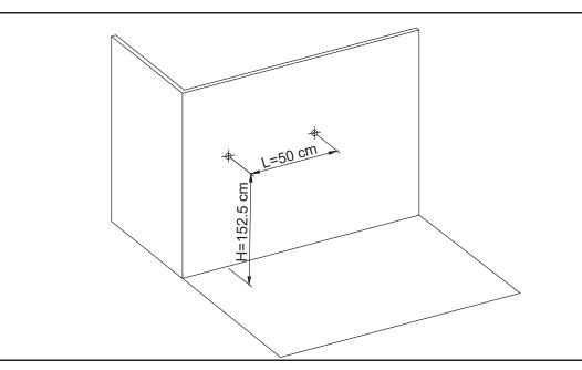
A : Determine the location where the screws should be inserted into the wall. Mark the point at the same height and lenght on the wall as shown above.
