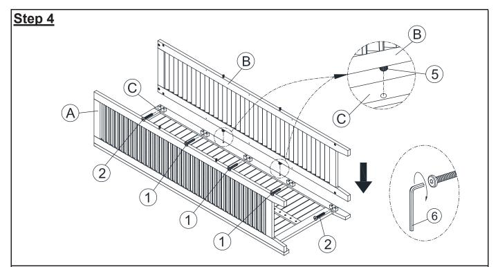
From step 3, Using the Allen Wrench (6), attach Side Panel Left (B) into assembly Back Panel (C) as shown above by using Bolts (2) and Screw (1). DO NOT: Fully tighten the bolts and Screw
