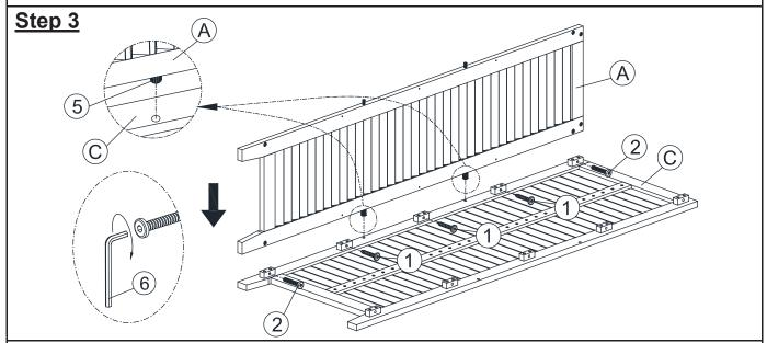
From step 2, attach Back Panel (C) to the Side Panel Right (A) to the wooden dowel position hole. Use Allen Wrench (6) to link the two panel with Bolts (2) and Screws (1). DO NOT: Fully tighten the bolts and Screw
