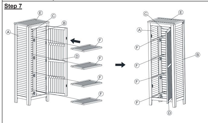
From step 6, Rotate the Removable shelf (F) to place it inside the cabinet. as shown in the above picture.
