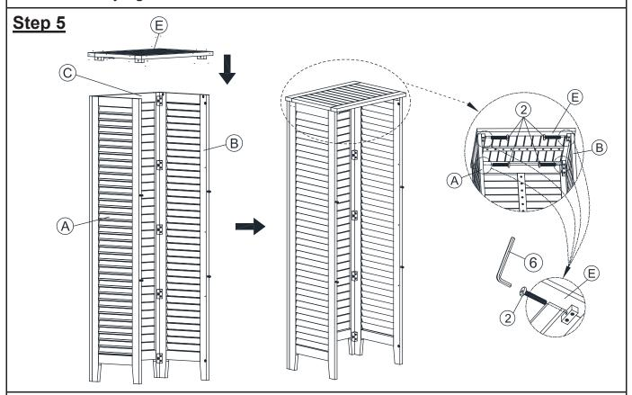
Stand up the assemble in step 4, then using the Allen Wrench (6), attach Top Panel (E) to the assembly in step 4 as shown above by using Bolts (2). DO NOT: Fully tighten the bolts
