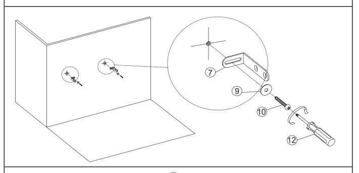
C: Affix the L-shaped Metal Bracket (7) to the wall.
