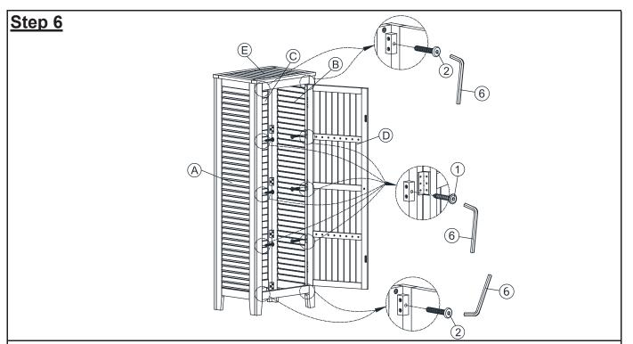
From step 5, Attach Door Frame (D) into the wooden dowel position hole. After open Door Frame. Next using Bolts (2) and screw (1) by Allen Wrench (6)In a sequential manner, gradully tighten all Bolts and Screws until evenlysecured
