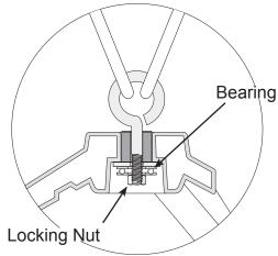
**Maintenence**: Periodically check that the Locking Nut on the bottom of the center of your spinning wheel is fully engaged. Every year the Stainless bearing should be lubricated with a light houshold oil or light grease. Too much grease will attract dirt. Wipe away any excess lubricant.
