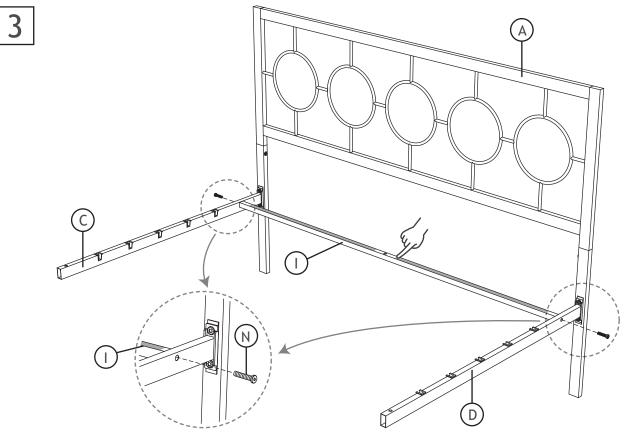
Note: Please make sure the adhesive strips are up when you install the metal beam I.
