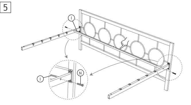
Note: Please make sure the adhesive strips are up when you install the metal beam I.
