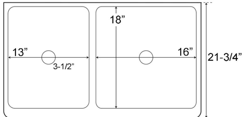
Dimensions of fixture are nominal and may vary within the range of tolerances established by ANSI Standard A112.19.2. Dimensions and specifications subject to change without notice.
