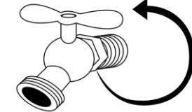
2) Wrap the tape around the threaded end of the spigot in a counterclockwise direction.
