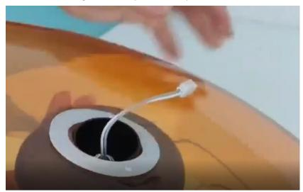
Step 6: Reconnect Wires Reattach the wires between the light head and body. Ensure connections are secure.
