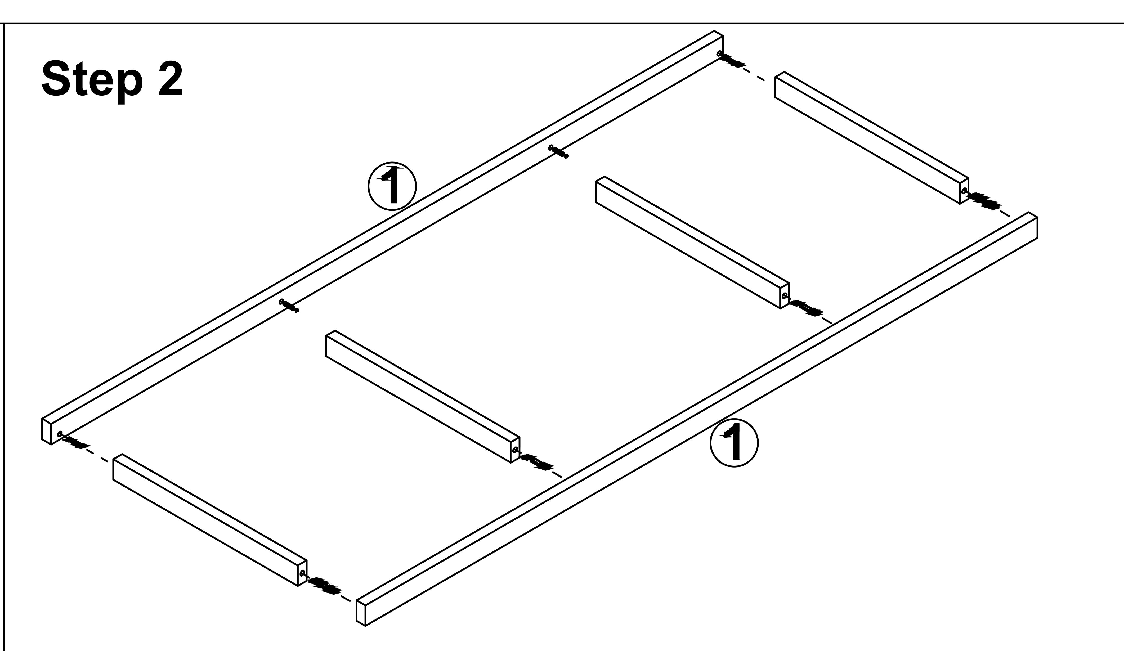
the 1# boards with the Four workpieces of Step 1. \*Note that there is a drilled hole under each triple connector, but the wooden tenon is not.
