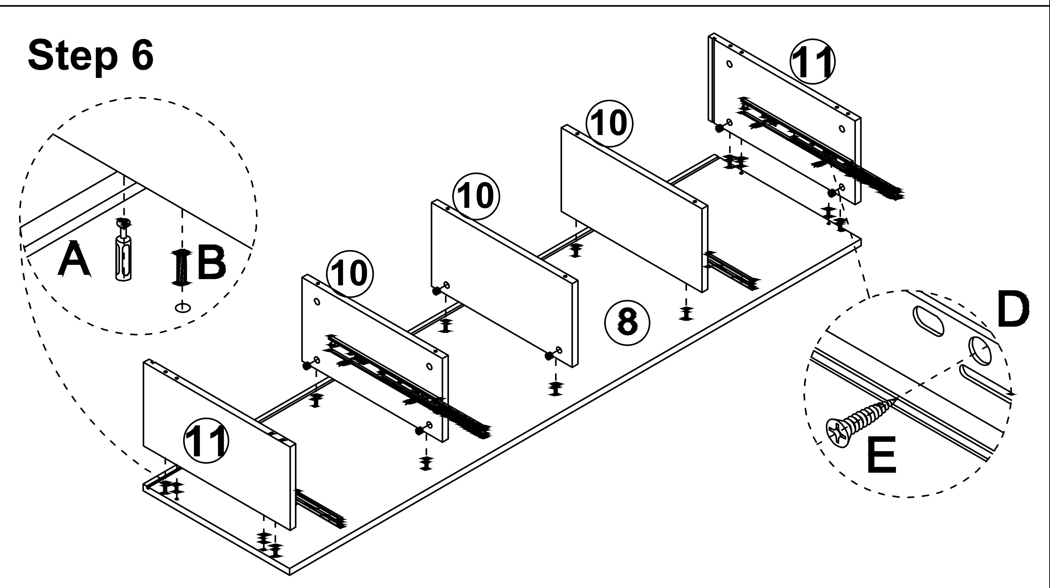
**Connectors (A) and Wooden Tenon (B). install the Slide Rails (D)** between the 10# and 11# boards with Self Tapping Screws (E)
