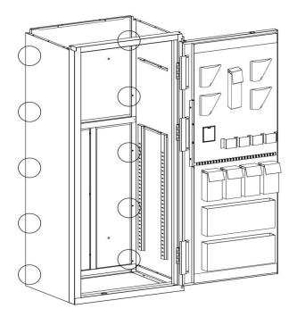
Install the back panel with 10 self-tapping screws.
