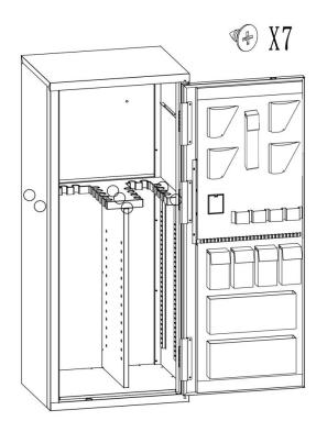
Install gunstock laminate, connect the two sides and center vertical plate with 7 self-tapping screws.
