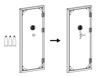
Rotate the handle once to secure it.Connect
