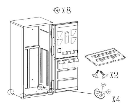
Install the bottom shelf, the front edge of the bottom plate hooks the front frame, and the remaining three sides are clamped into the sides and back, It is fastened with 4 E-type metal parts and 8 screws
