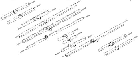
Step 2: Attach the 1 x back left corner panels(15) and the 1 x front left corner panels (2) to the 1 x Bottom head rail (3), 1 x Top head rail (11) and 1 x Head Panel (12) using hardware parts (A) and (C). Then attach the 1 x Back left roof panel (4) and 1 x front left roof panel (5) using hardware part (B). DO NOT use any power tools as this may damage the frame and will invalidate any claim.
