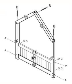
Step 3: Attach the 1 x Front right corner panels (1) and the 1 x Back right corner panels (16) to the 1 x Bottom head rail (3), 1 x Top head rail (11) and 1 x Head Panel (12)using hardware parts (A) and (C). Then attach the 1 x Back right roof panel (6) and 1 x front right roof panel (7) using hardware part (B).
