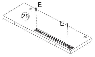
Fix rail(D-CR) to panel 28 with screw(E) as shown. **Flip to back,** fix rail(D-CL) as shown.
