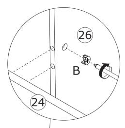
Attach the two components to panel 24, add cam lock(B) into and turn clockwise to tighten as shown.
