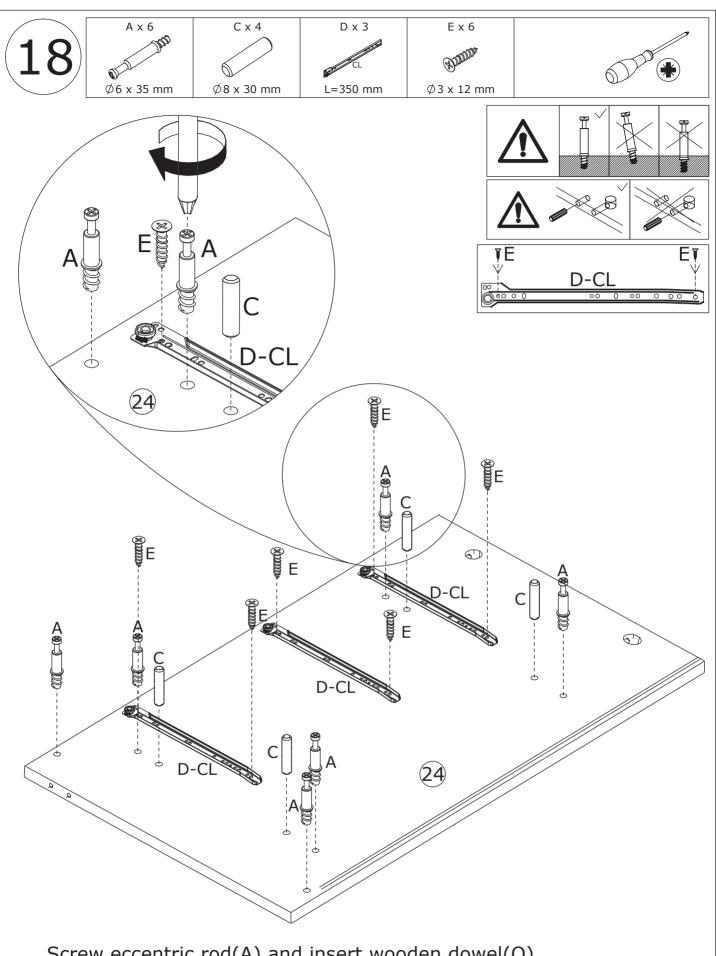
Screw eccentric rod(A) and insert wooden dowel(Q) into panel 24 at first.
