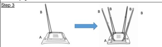
Repeat Step 2 to assemble the remaining legs using Bolts(1), Spring Washers(3) and Washers(2) with the Allen Wrench(5).
