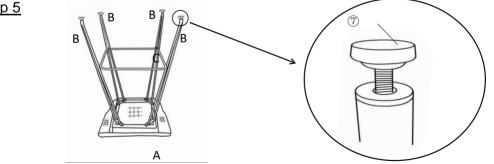
Install the Leveller( $\odot$ ) into the bottom of the Chair Leg(B), tighten by turning the Leveller clockwise.
