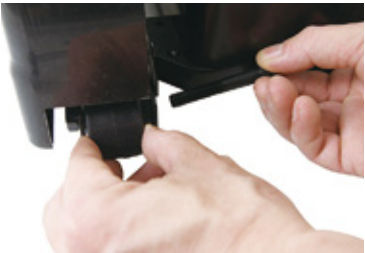
Use screws to install left bottom wheel.
