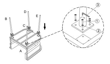
Keep the bolts loosen while setup and tight all the bolts until the legs have already in place.
