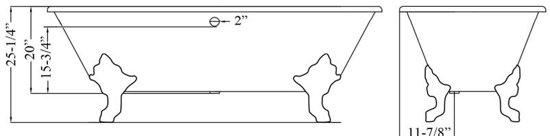
Dimensions of fixture are nominal and may vary within the range of tolerances established by ANSI Standard A112.19.2. Dimensions and specifications subject to change without notice.
