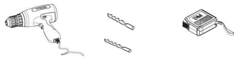
Electric drill Drill bit (Φ8/Φ5) Tape measure (3m~5m)
