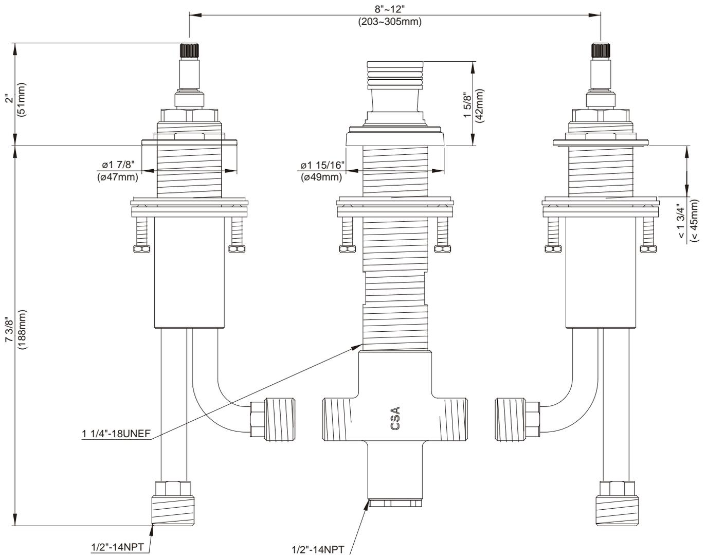
\* Installation method shown is for deck thickness of less than 1-3/4".
