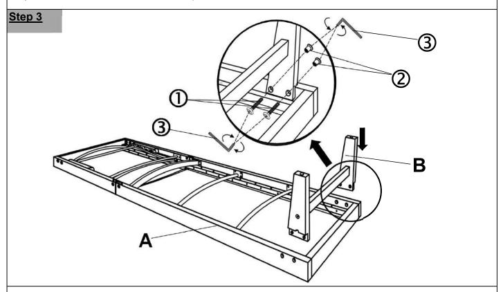
Attach Leg frame (B) to Foldable seat panel (A) by using Bolt (1), Sleeve nut (2) and Allen Key (3) as shown in picture above.
