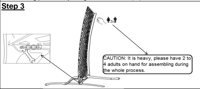
Hold the Seat Panel(B) up and align the mounting positions to the Bolts(3) on the Left Armrest(C).
