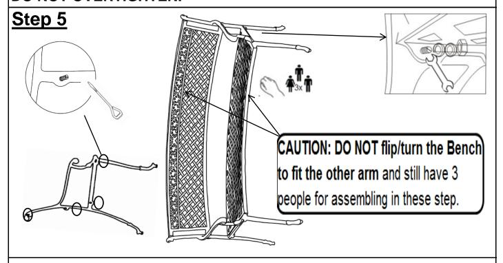
Lock four M8\*40mm Bolts(③) into the mounting positions of the Right Armrest(D) the same as you did in Step 1.
