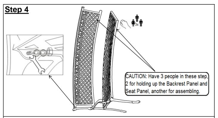
Hold the Backrest Panel(A) up and align the mounting positions to the two Bolts(③) on the Left Armrest(C).
