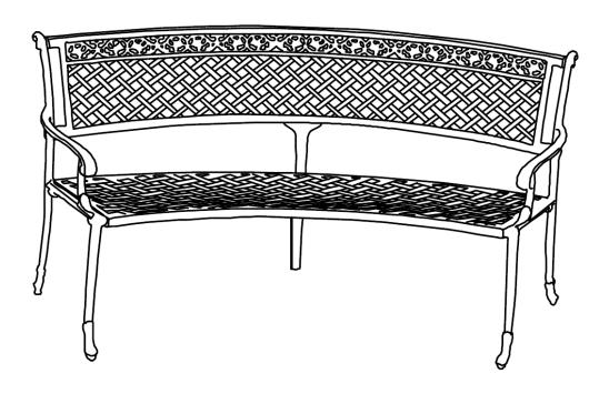
Adjust the Pre-installed Rubber Levelers on the Legs until the Bench is level to the ground.
