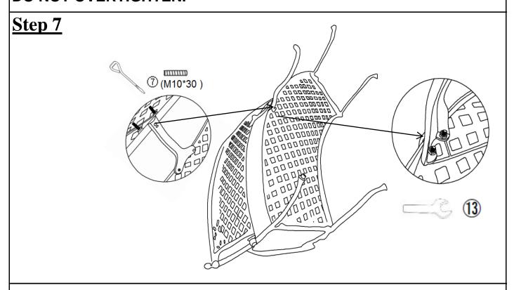
Lock two M10\*30mm Bolts( $\bigcirc$ ) to the underside of the Seat Panel(B) by using the Screwdriver( $\bigcirc$ ).
