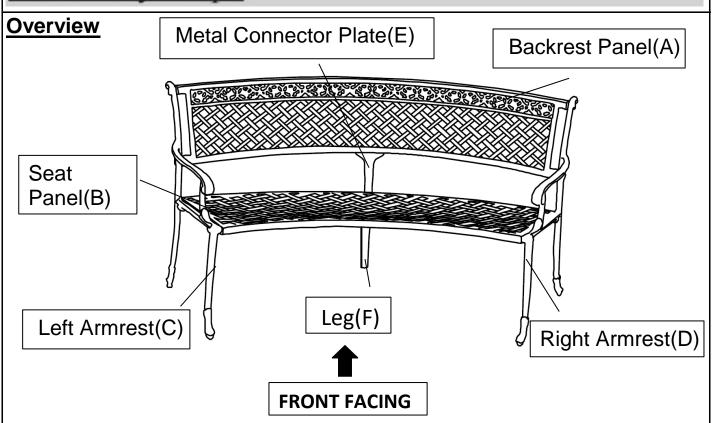
This Bench has multiple parts and may require up to some 30 minutes to assemble. To give you an overview of the Chair parts, the above picture is to help you put the various parts into perspective. Please read through the instructions herebelow to familiarise the parts and steps before assembly.
