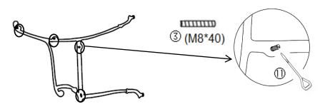
Place the Left Armrest(C) on the floor and lock four M8\*35mm Bolts(③) to the mounting positions by using the Screwdriver(①).
