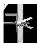
3.Tighten screw until flush with item.
