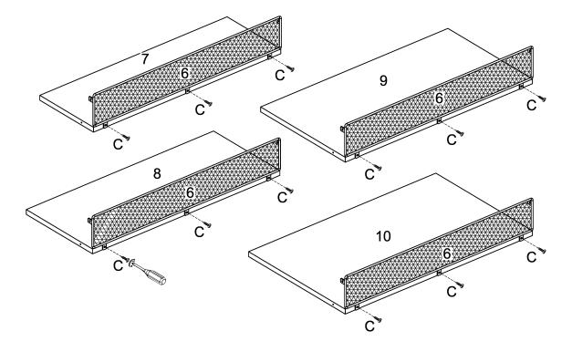
Attach parts (6) to parts (7,8,9,10) using screw (C) and a Philips Head screwdriver as per diagram .
