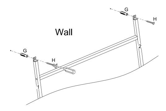
Using screw (H) insert parts (1,2) to anchor (G) with Philips Head screwdriver as per diagram.
