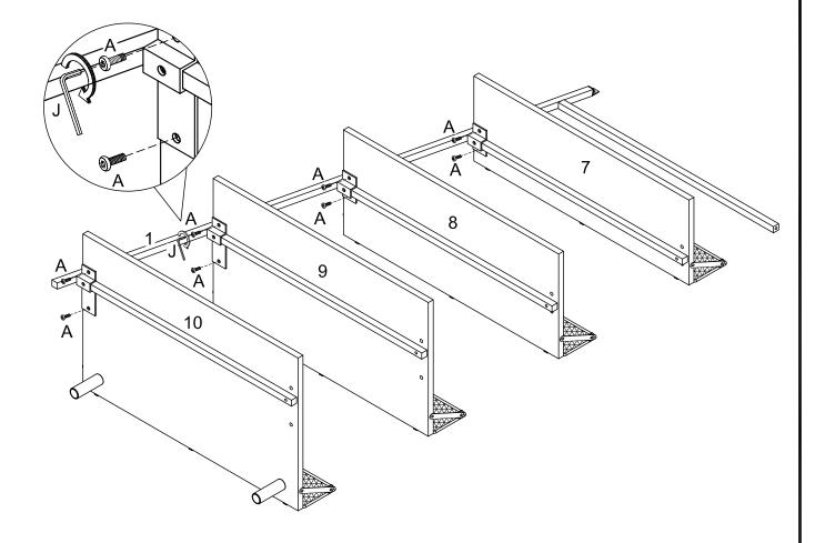
Using bolt(A,B) attach parts (7,8,9,10) into part (1) with hex key (J) as per diagram.
