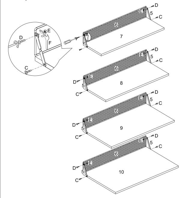
Attach parts (5) to parts (6) and parts (7,8,9,10) using bolt (D), Wrench (F) and Philips Head screwdriver as per diagram.
