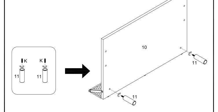
Insert bolt (K) to part (11) secure to part (10) as per diagram.
