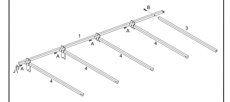
Use bolt (B) to attach part (3) to part (1). Then use bolt (A) to attach part (4) to part (1) as per diagram.
