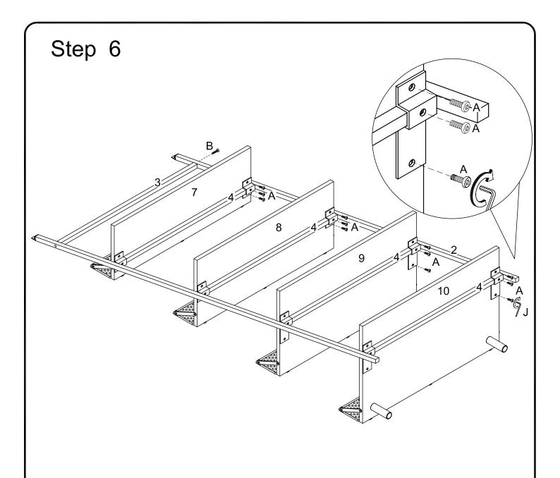
Using bolts (A,B) secure parts (3,7,8,9,10) into part (2) with hex key (J) as per diagram.
