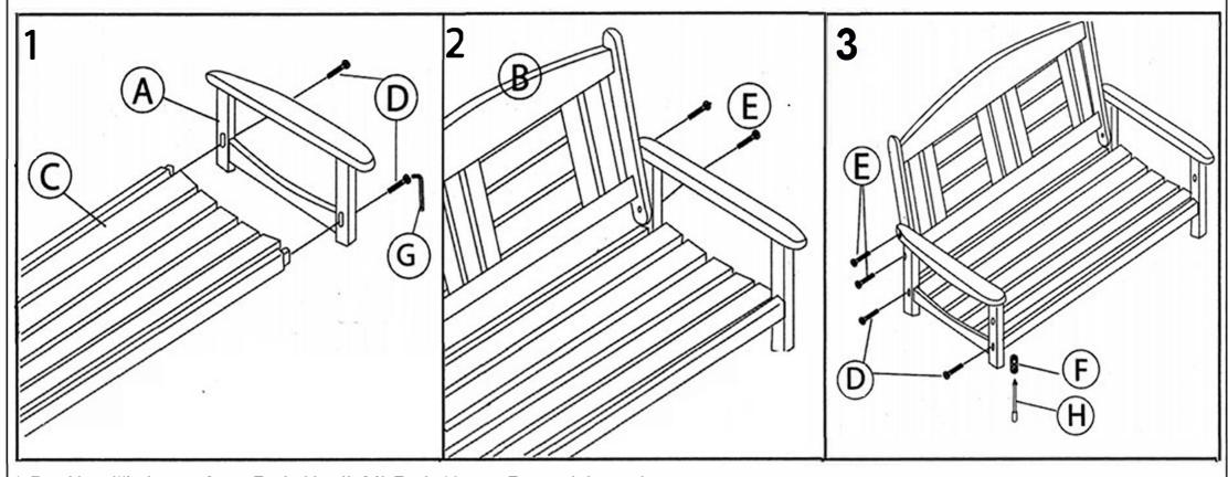
\* Do Not Tighten Any Bolt Until All Bolt Have Been Placed.
