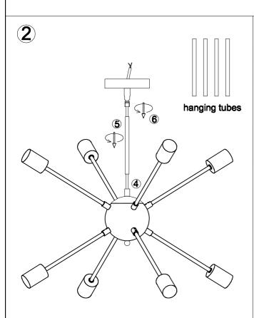
2.Let the wire go through the hanging tube5 and the base6, turn to fasten the hanging tube5 on the ball and the base.
