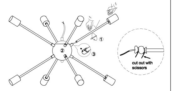
1.Turn and fix the tube1 on the ball2, lock it with screw3. (note: please hold the tube not the cup by your hand when install the tubes.)
