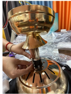
Step 9: The hole on the boom matches the hole on the main body, and the pin is fixed with the R pin on the other side through the hole
