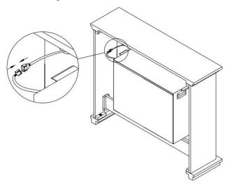
5.6a Install fire from the back of mantel, use 4pcs ST4×12 screws to fix insert to mantel.
