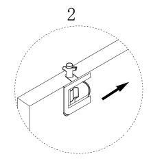
Align the cross shape of fastener  ${}^{\prime\prime}B{}^{\prime\prime}$  on the vertical plate with the hole position on the top plate and bottom plate,
