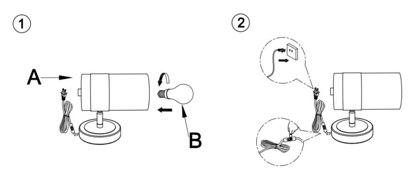
Step 1:Remove lamp body(A) from the packaging box and install light source(B) light source on lamp body(A). Put the light on a level surface to check if everything is stable.
