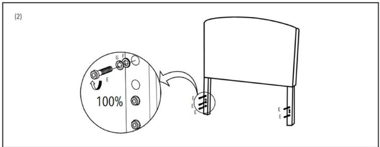
Ensure that all bolts are tightened before use. Check and tighten all bolts periodically throughout use of the product.
