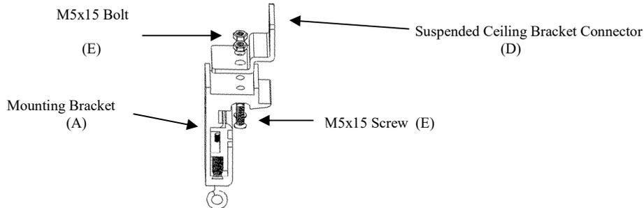
3. Insert chains (not included) through the loop holes of the **Suspended Ceiling Bracket Connector(D)**.
