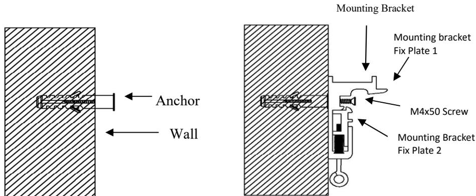
3. Attach the screen to the **Mounting Brackets (A)** by inserting the top of the case to Fix Plate 1 and securing the back of the case to Fix Plate 2. Make sure the case slots are securely attached to the mounting brackets.
