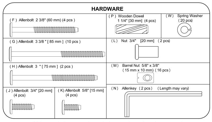
Make sure the bolts are tightly locked against the washers during assembly. (Please add an extra ½ revolution to all the bolts when using spring washer after tightening)
