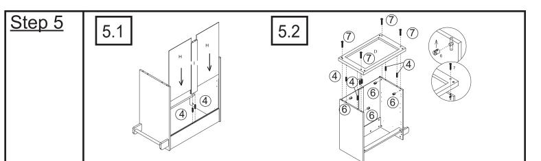
5.1)Insert Down Back Board(H)and into the mounting positions on UP Back Board(J)
