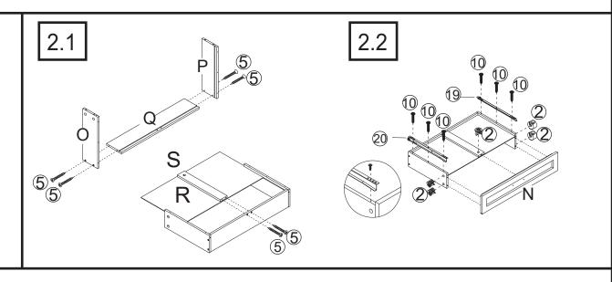
2.1)Attach Drawer Left Panel (O)and Drawer Right Panel (P) to the Right Side Panel (Q) with Screw (5)
