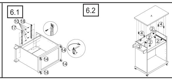
6.1)Attach Left Guide Rail (7) to the Left Side Panel (G) with Screw (10)
