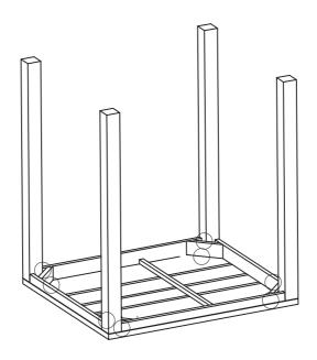
Tighten all 8 Screws into place with Allen Key (F)
