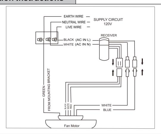
**NOTE:**Once earth wires are connected, carefully tuck all wires and marrettes into the meta box making sure that the wires are clear of the hemisphere and downrod when positioned in hemisphere and downrod when positioned in mounting bracket.
