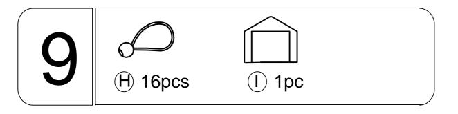
Fix the Front tarp (I) and Top tarp (D), Front tarp (I) and Tarp wall (K) by Elastic band (H).
