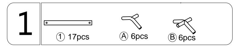
Put Top tube (1), Three-way tube joint (A) and Four-way tube joint (B) in the shown order.
