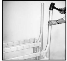
**Step 4:** Using a rubber mallet, install the four handrail posts into the middle slots of the top two step locations on the left sidewall, and the top two step locations of the right sidewall. Handrail posts must be seated into the slots
