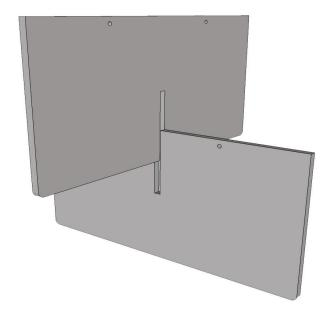
**Step 1:** Assemble **Legs** together by sliding the cutout of one into the cutout of another. Sides of legs with holes should be the higher hoizontal edge for the next step.
