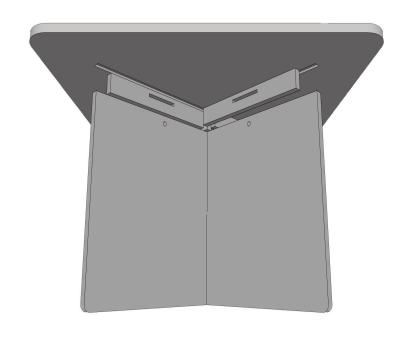
**Step 2:** Place **Table** on top of leg assembly. Align dados in underside of Table with edges of leg pieces. Sides of legs with holes should be closest to the underside of table. Do not attempt to move cleats on underside of table.
