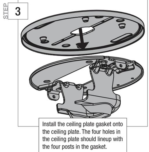
Install the ceiling plate gasket onto the ceiling plate. The four holes in the ceiling plate should lineup with the four posts in the gasket.
