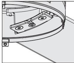
Insert the blade into the blade slot around the center screw. Put the blade washers found in the ■ hardware bag onto the blade screws found in the ▲ hardware bag. Then install the blade screws to secure each blade to the fan.
