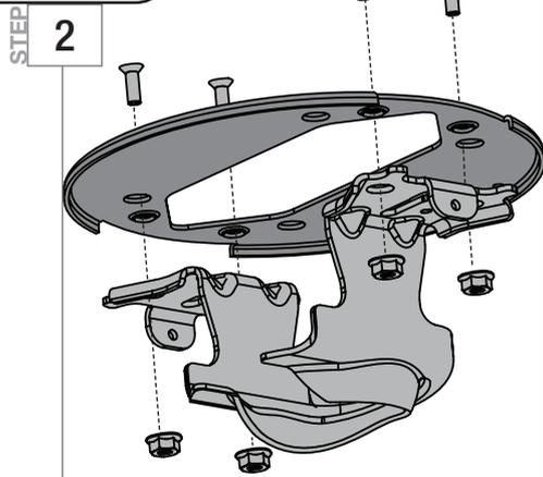
Align the tapered mounting holes in the ceiling plate with the holes in the ceiling bracket. Install the four ceiling plate screws found in the hardware bag and secure with the flange nuts using an 11/32" wrench. Hold the ceiling bracket assembly up to the outlet box and mark the screw locations. To mount to support structure, also mark the ceiling for drilling pilot holes.
