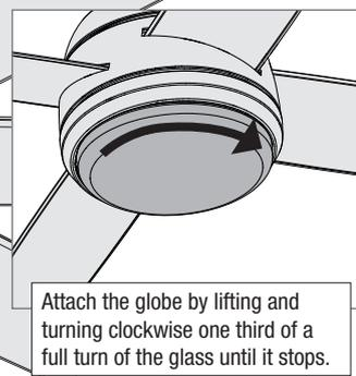
Attach the globe by lifting and turning clockwise one third of a full turn of the glass until it stops.
