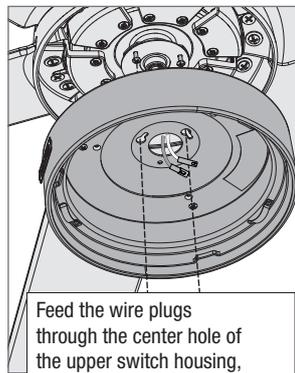
Feed the wire plugs through the center hole of the upper switch housing, then wrap keyhole slots around the screws and twist counterclockwise.
