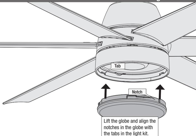
Lift the globe and align the notches in the globe with the tabs in the light kit.
