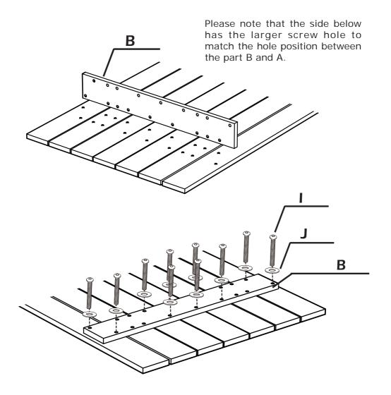
For the hole position, please leave an appropriate gap between the part A and A1.
