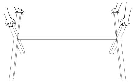
If you find the part C and D are unstable after installation, please stand the table legs on a flat bottom surface as shown and press downward.
