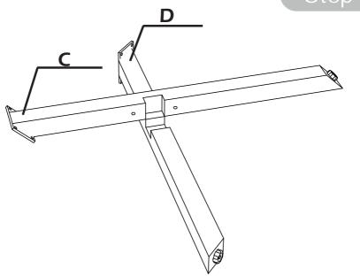
Please put together the 4 legs in an "X" shape according to the number then turn it over to the reverse side and prepare to install part E with screws.
