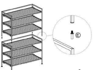
Build a second shoe rack and screw the STACKING PINS (E) into the legs of the FRAME (A) instead of the feet.
