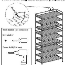
After stacking more than 2 units high, wall mounting is required for safety.
